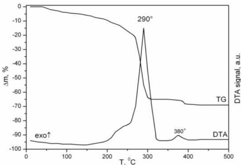
Figure 3. TG and DTA curves of sample Cr12PG synthesized at 130°C
