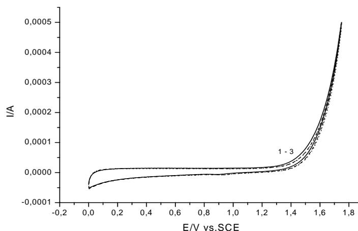
Fig. 2. Cyclic voltammogram of Ti/SnO<sub>2</sub>-Sb<sub>2</sub>O<sub>5</sub> in 0.1 M Na<sub>2</sub>SO<sub>4</sub>; three repeated scans; scan rate 0.05 V/s; potential range: 0 V to 1.75 V vs. SCE; 1- first repeated scan; 2-second repeated scan; 3-third repeated scan
