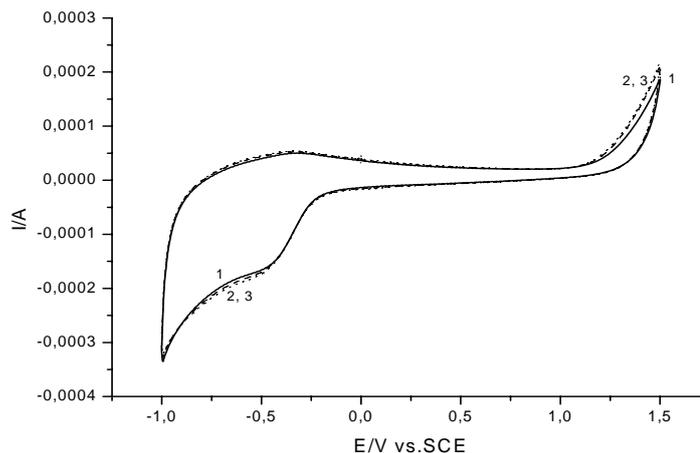
Fig. 3. Cyclic voltammogram of Ti/SnO<sub>2</sub>-Sb<sub>2</sub>O<sub>5</sub> in 0.1 M NP6EO 0.01 g/L in 0.1 M Na<sub>2</sub>SO<sub>4</sub>; three repeated scans; scan rate 0.05 V/s; potential range: -1.0 V to 1.5 V vs. SCE; 1- scan in the presence of Na<sub>2</sub>SO<sub>4</sub>; 2-scan in the presence of NP6EO 0.01 g/L in 0.1 M Na<sub>2</sub>SO<sub>4</sub>; 3- repeated scan in the presence of NP6EO 0.01 g/L in 0.1 M Na<sub>2</sub>SO<sub>4</sub>
