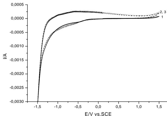
Fig. 1. Cyclic voltammogram of Ti/SnO<sub>2</sub>-Sb<sub>2</sub>O<sub>5</sub> in 0.1 M Na<sub>2</sub>SO<sub>4</sub>; scan rate 0.05 V/s; potential range: -1.5 V to 1.5 V vs. SCE; 1- first scan; 2-second scan; 3-third scan
